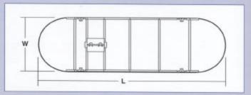
flexibility in locating mounting boxes, and provide for rigid placement during installation. End sections are radiused on state-of-the-art CNC equipment and include the same 1-1/4" bottom flange as the straight sections ... a Red-E-Form exclusive. All knocked-down sections are now supplied with the revolutionary **Red-E-Flange** stamped steel flange for the best fit in the industry. Forms are prime coated and supplied with the essential hardware for fast assembly.
