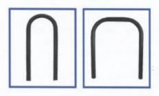
**Pipe Guards:** Red-E-Form® pipe guards are designed to provide maximum protection for valuable island equipment and are available in several styles. Pipe guards are fabricated from one continuous piece of Sch. 40 pipe with 12' radius bends. Pipe is available in 3-1/2" OD or 4" OD, painted with one coat of metal primer. Stainless steel pipe guards are available in 3-1/2" OD with a 180 grit polished finish. 6' and 8" Sch. 40 straight pipe are also available.
