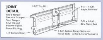
Permanent Steel Island Forms: All Red-E-Form permanent steel island forms are fabricated from high quality 12 ga. steel. Sections are precision roll formed, providing unsurpassed dimensional accuracy and eliminating many installation problems often found in standard knocked-down forms. Standard 1-7/8' rolled top bead and 1-1/4' bottom return flange provide strength and accurate alignment. Double cross bracing and adjustable top braces allow
